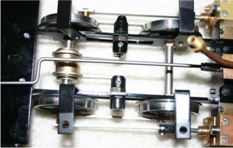
Using a 1.5 mm hex key, screw a stainless set screw into the hole in the inside rocker arm. The photo shows set screws protruding from both rocker Arms.
