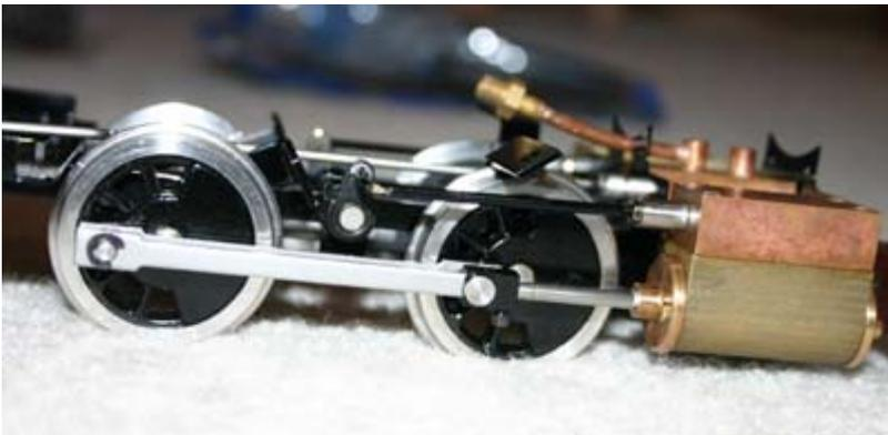
Beginning with the right side of your engine (shown in photo) rotate the drivers until the side and valve rods are at rear dead center as shown in the photo. Note that the side and valve rods are parallel with each other. Without changing the position of the drivers, turn your engine upside down.
