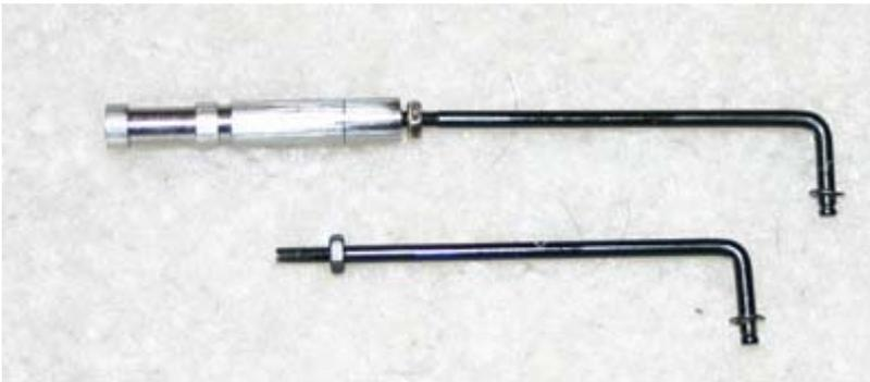
In the short leg of each valve rod are two grooves. Place a small E-clip on each inside groove. This is a very fiddley job. What worked best for me is to use a large set of needle nose pliers to push the E-clip onto the rod.
