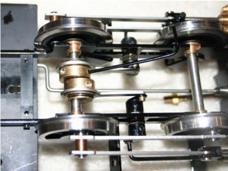
Insert a set screw in the eccentric and screw it in with a 1.5 mm hex wrench until it is nearly tight.
